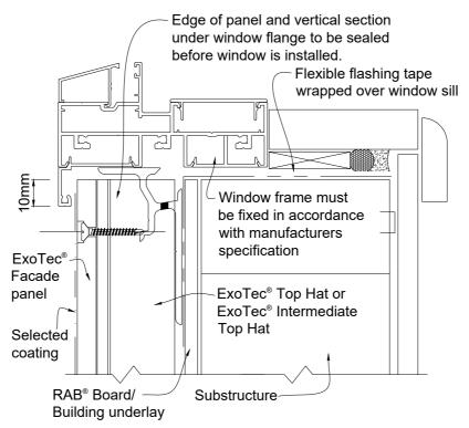
Note: When RAB® Board is used with timber frame flashing tape to be applied to the entire window opening
